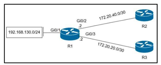
Which configuration configures a policy on R1 to forward any traffic that is sourced from the 192.168.130.0/24 network to R2?
