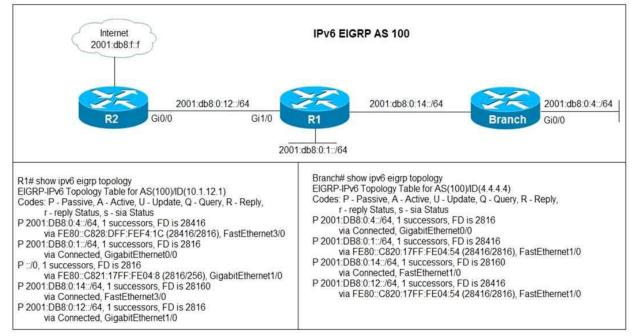
Users in the branch network of 2001:db8:0:4::/64 report that they cannot access the Internet. Which command is issued in IPv6 router EIGRP 100 configuration mode to solve this issue?
