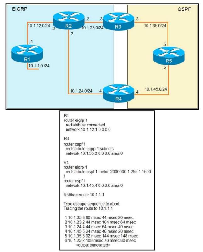
The output of the trace route from R5 shows a loop in the network. Which configuration prevents this loop?
