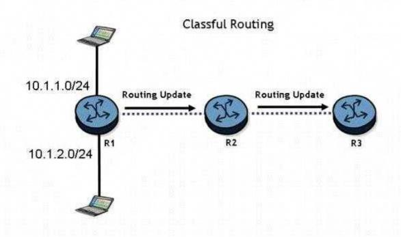
Routers R1 " R2, and R3 are running a classful routing protocol between them. Assuming that router R1 advertises all directly connected networks, how will these networks be represented in router R3's routing table?
