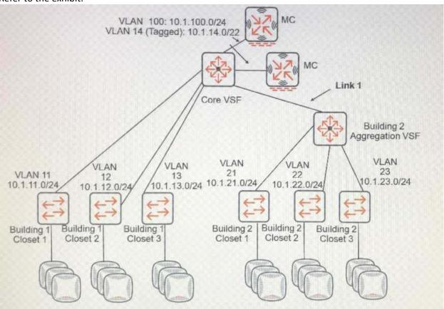
The customer needs to expand its wired and wireless network to a new building, Building 2, which is near the existing building, Building 1. The exhibit shows the logical plan that the architect has created so far. The aggregation layer switches in the new building should provide the default gateway services for the VLANs in the new building and route traffic to the core. The existing Aruba Mobility Controllers (MCs) will control the new APs.
