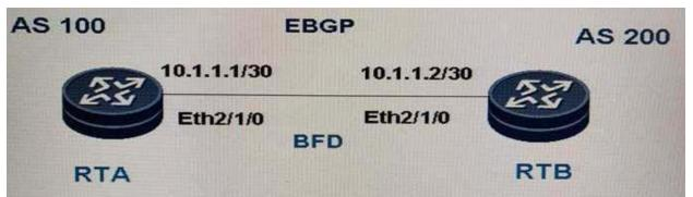
As shown in the figure, RTA and have one BGP session. To detect fault fast, the BFD for BGP feature needs to be configured on RTA and RTB. BGP-related configurations are as follows:
